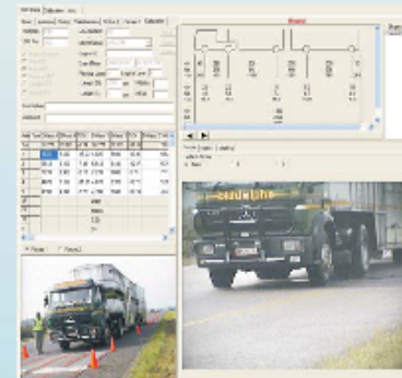
Output from the calibration module providing video confirmation of calibration vehicles used at both the HSWIM and reference scales
